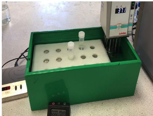
**FIGURE 3** Samples (~0.5 g) in 40 ml, 30 × 84 mm polypropylene tubes in a designed polypropylene tube holder (Megazyme cat. no. D-PPTH) [C (w)] on a 2mag Mixdrive 15® submersible magnetic stirrer in a custom-made water bath (Megazyme cat. no. D-TDFBTH). This arrangement allows stirring of 15 samples at controlled speed (170 rpm) and 37°C [Color figure can be viewed at [wileyonlinelibrary.com](http://wileyonlinelibrary.com)]
