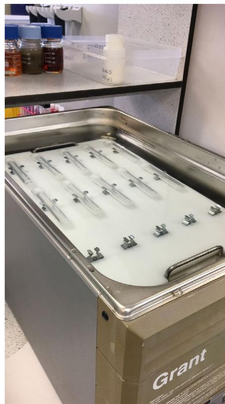
**FIGURE 1** Attachment of 13-ml polypropylene tubes to a polypropylene tube holder in a Grant OLS 200 water bath [Color figure can be viewed at [wileyonlinelibrary.com](http://wileyonlinelibrary.com)]
